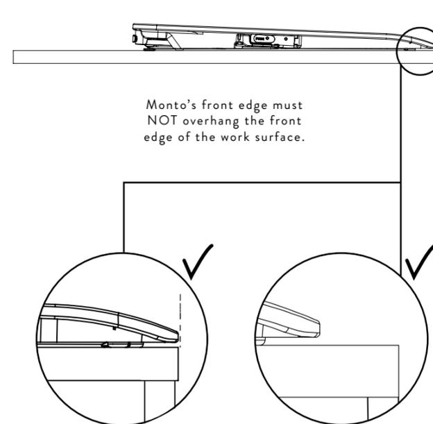
Monto's front edge must NOT overhang the front edge of the work surface.
