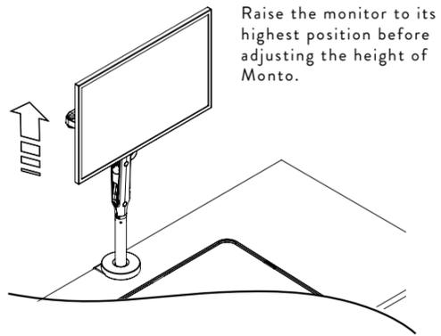
3.2 RELEASE THE MECHANISM AND ADJUST
