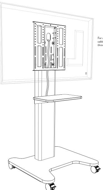
For a tidy installation, feed equipment cables up behind screen mount and through the cable management hole.
