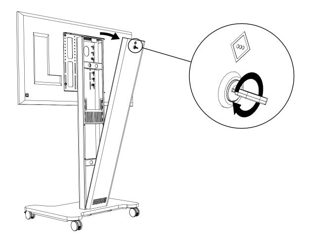
POSITION COLUMN BRACKET ON THE INSIDE OF THE COLUMN
