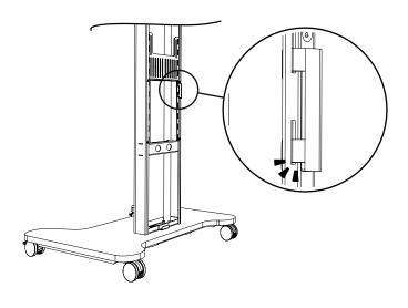
3.4 INSTALL SHELF TO COLUMN USING THE SAME 'HOOK ON' INSTALLATION METHOD
