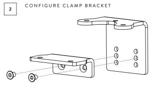
If required change the clamp plate setting by removing Countersunk screws and adjusting to correct setting
